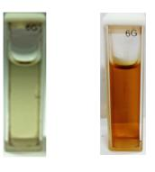
(a) (b) **Figure 1.** Photographs of the colloidal chitosan-AgNPs: (a) before and (b) after heat treatments.
