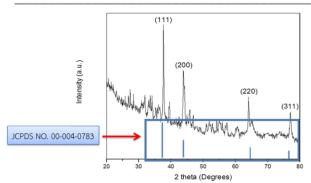
Figure 6. XRD patterns of the colloidal chitosan-AgNPs.
