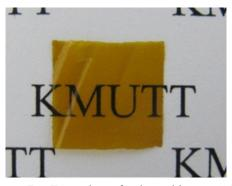
**Figure 7.** Example of the chitosan-AgNPs composite transparent film fabricated by casting method on the glass plate.
