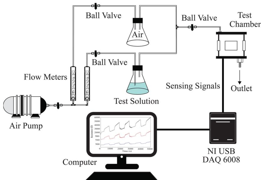
Fig. 4 Schematic illustration of standard flow-through system for gas sensing measurements at room temperature.
