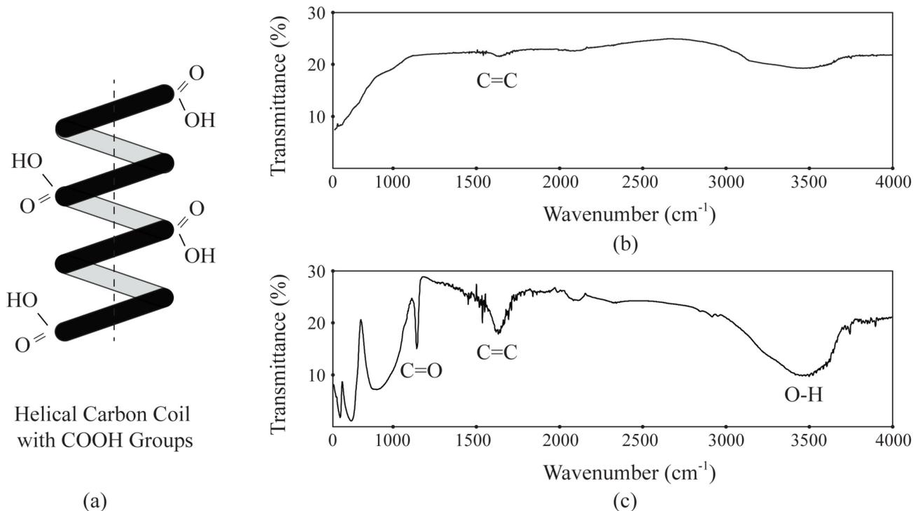
Fig. 2 (a) Schematic illustration of modification for helical carbon coil with COOH groups, FTIR spectra of (b) as-grown helical carbon coils and (c) purified helical carbon coils.
