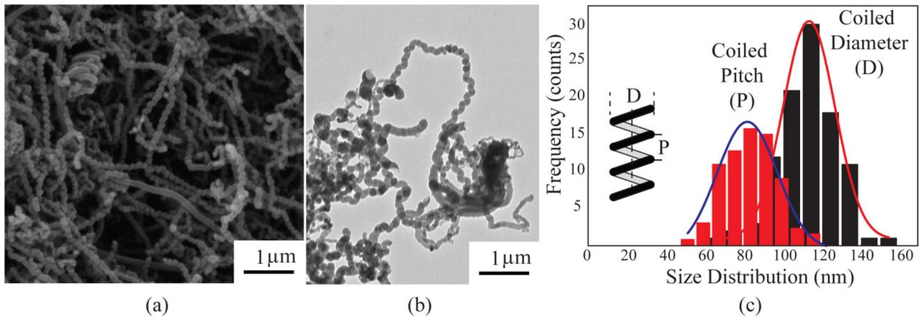
Fig. 1 (a) SEM, (b) TEM images and (c) size distribution of as-grown helical carbon coils.
