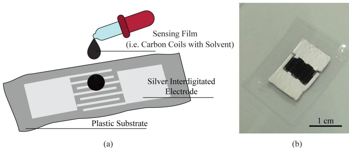
Fig. 3 (a) Schematic illustration and (b) photograph of helically coiled carbon gas sensor.
