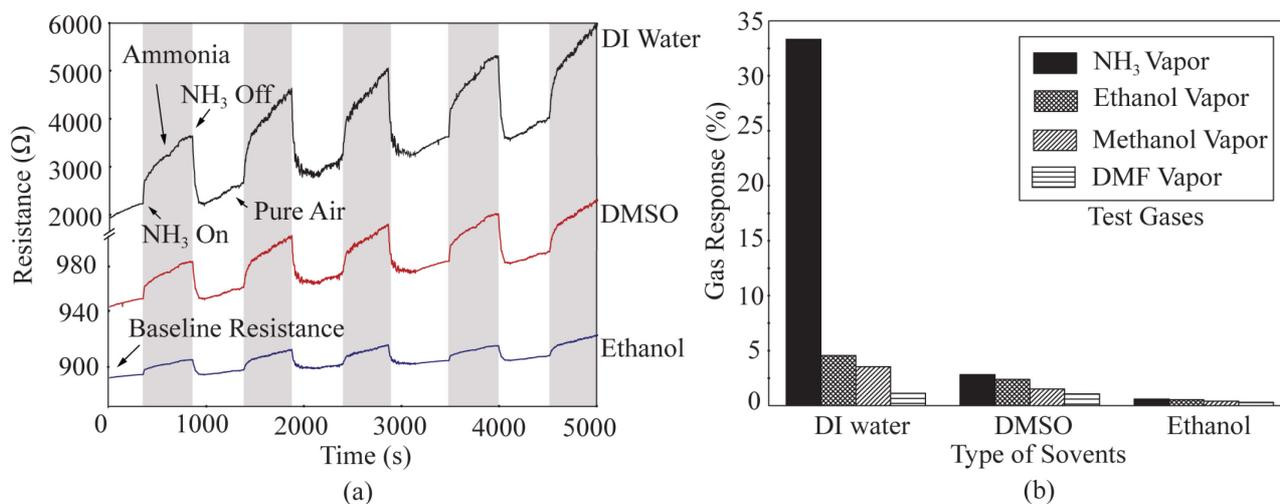
Fig. 5 (a)  $\text{NH}_3$  sensing behavior and (b) gas response of fabricated as sensor at room temperature.
