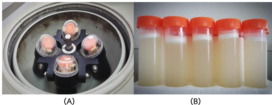
Figure 1 Latex serum separated by using centrifugation techniques (A) and centrifuge bottle (B); latex particle (top) and latex serum (bottom)
