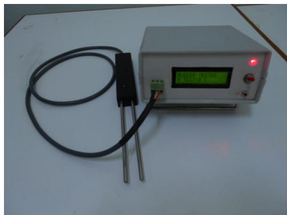
Figure 6 The designing and constructing of Fresh Latex Quality Measurement Machine prior testing
