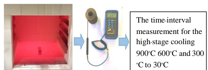
Figure 4 Burning in furnace and measurement of cooling rate of the finned tube.
