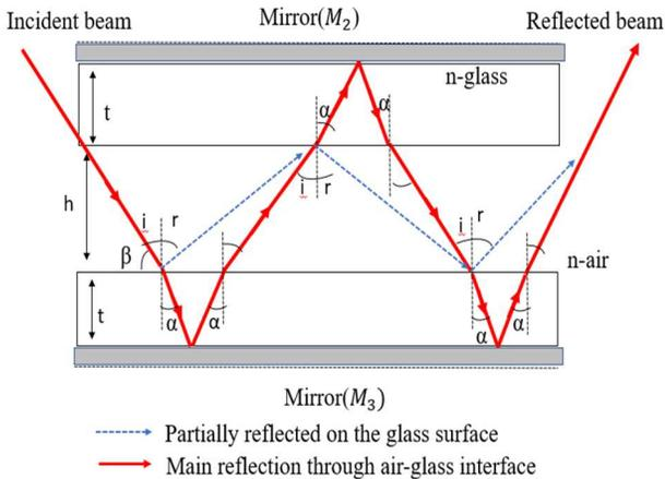
Fig. 2. Schematic of the multiple reflections between the two mirrors  $M_2$  and  $M_3$ .
