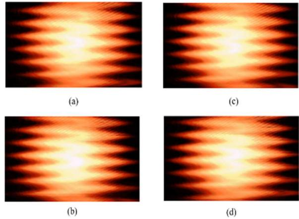
Fig. 3. An interferogram captured at the phase shift of (a)  $0^\circ$ , (b)  $90^\circ$ , (c)  $180^\circ$  and (d)  $270^\circ$ .
