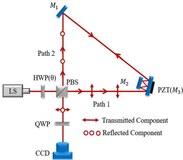
Fig.1. Schematic of the multiple reflections using modified Sagnac interferometer
