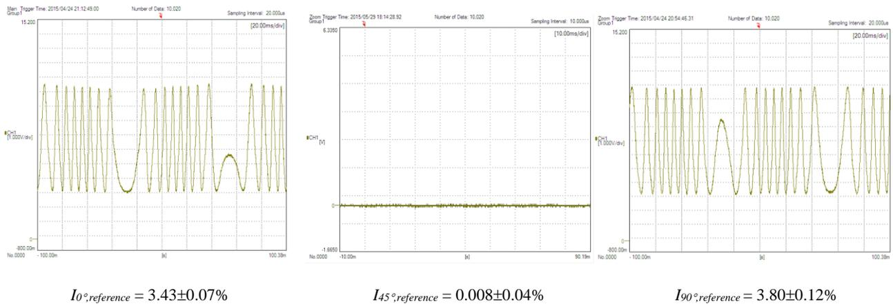
Figure 5. The intensity waveforms taken from an oscilloscope when HWP is oriented at 0°, 45° and 90°.
