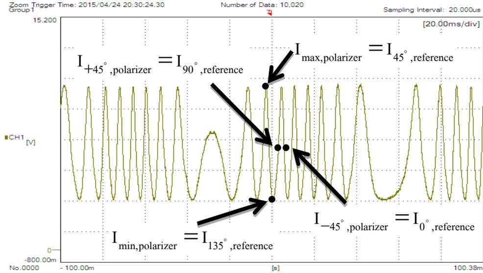
Figure 2. The experimental waveform signal taken from the oscilloscope and the intensity components at various output light orientations.
