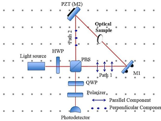
Figure 1. The schematic diagram of the polarizing triangular cyclic interferometer setup
