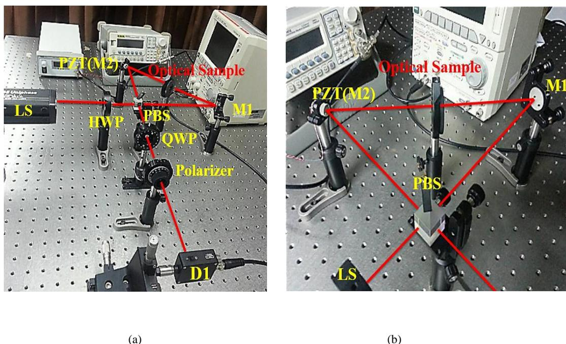
Figure 3. The photograph of (a) the complete arrangement of the polarizing triangular cyclic interferometer (b) the triangular cyclic part with inserted optical sample.
