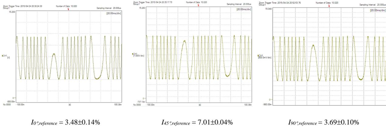
Figure 4. The intensity waveforms taken from an oscilloscope when QWP is oriented at 0°, 45° and 90°.
