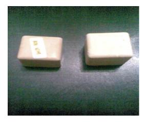
Fig 2. Rice Husk Ash Based Geopolymer
