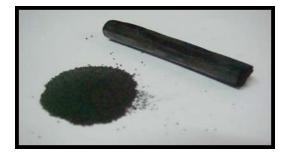
Fig.2 Photograph of carbon beads and carbon monolith
