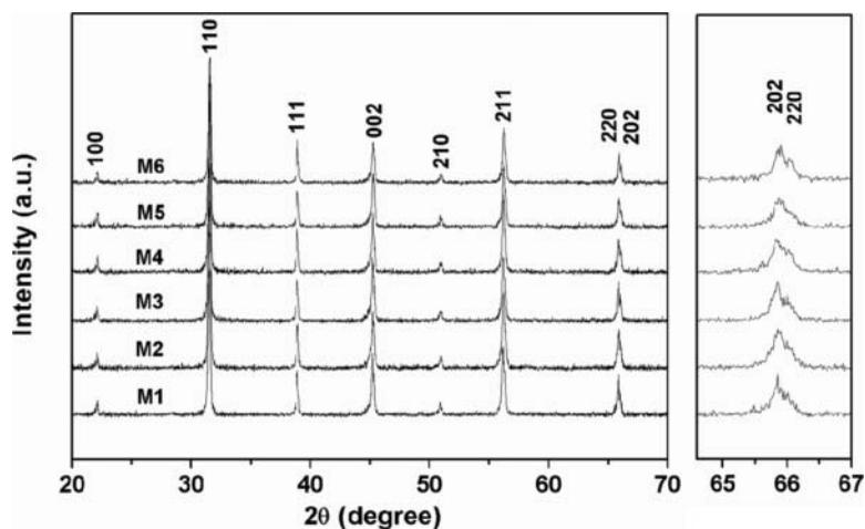
**Figure 1.** XRD diffraction patterns of the sintered ceramics.
