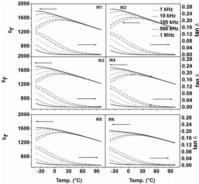
**Figure 4.** Dielectric constant and dielectric loss as functions of temperature for Mn and Sr doped content for BCZT-BZT ceramics.
