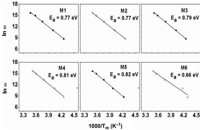
**Figure 5.** Plot of  $\ln(\omega)$  as a function of  $1000/T_m$  for the sample of BCZT-BZT ceramic dope with mol% Mn and Sr (symbols: experimental data; solid line: Eq. 1 fits).
