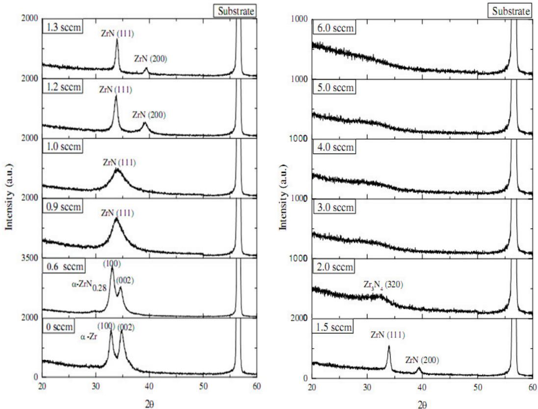
Fig. 3. X-ray diffraction patterns for Zr-N films deposited with various N<sub>2</sub> flow rates at Zr current of 0.6 A and deposition time of 15 minutes
