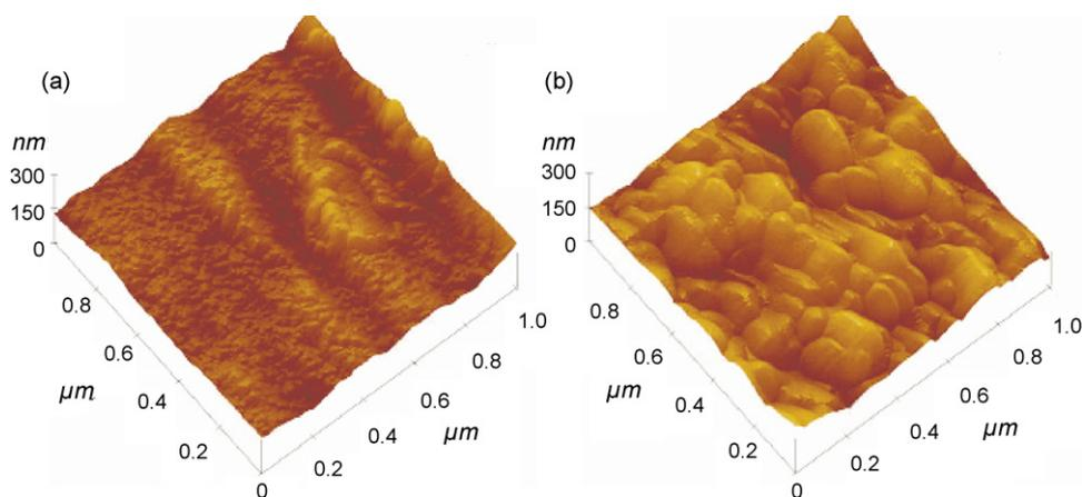
Fig. 9. AFM images  $2 \times 2 \mu\text{m}$  of silk fabrics. (a) before plasma treatment and (b) after plasma treatment at a  $\text{SF}_6$  pressure of 0.5 Torr, and RF power of 50 W for 5 min
