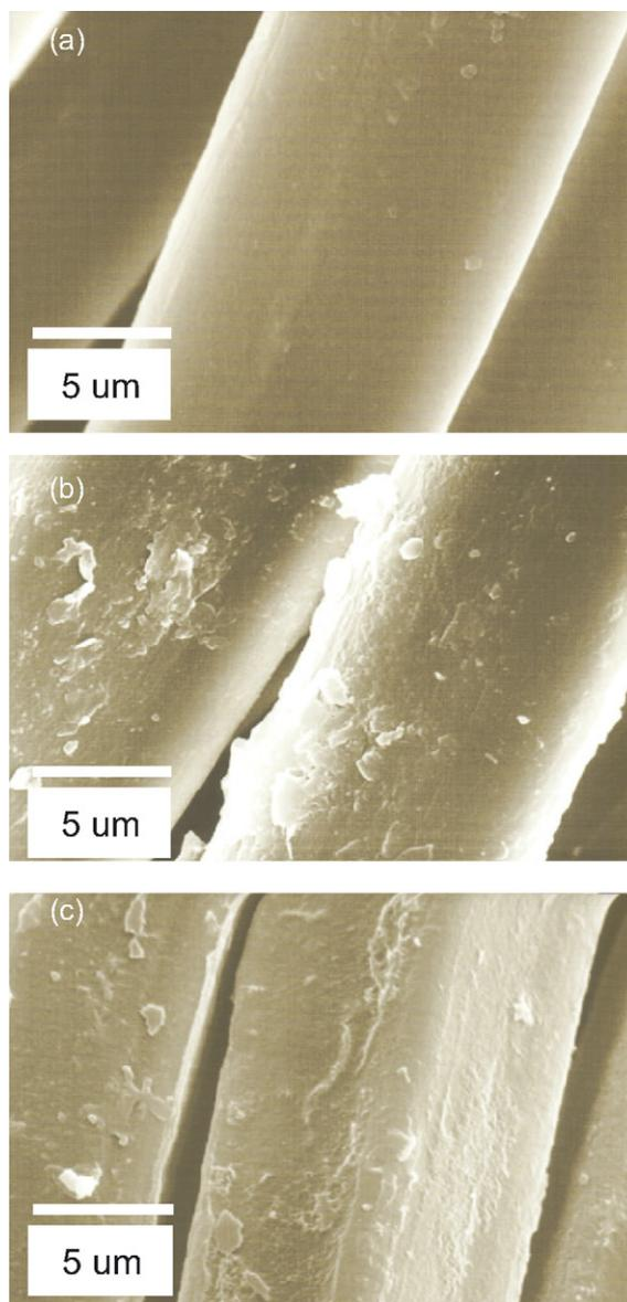
Fig. 8. SEM micrographs of silk fabrics with magnification of 3000. (a) Before treatment, (b) after treatment with 0.05 Torr of  $\text{SF}_6$ , and RF power of 25 W for 1 min and (c) after treatment with 0.5 Torr of  $\text{SF}_6$ , and RF power of 50 W for 5 min
