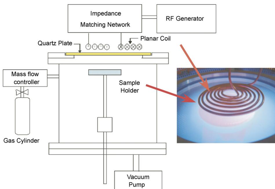
Fig. 1. Diagram of the radio-frequency (RF) inductively coupled  $\text{SF}_6$  plasma reactor.
